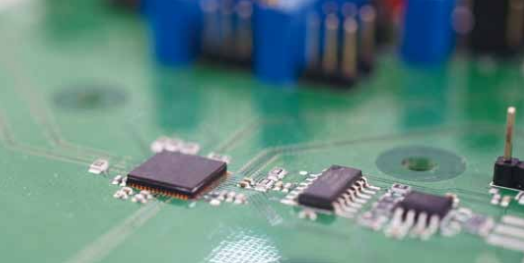
07 Test PCB with imec and Holst Centre's wake-up receiver
