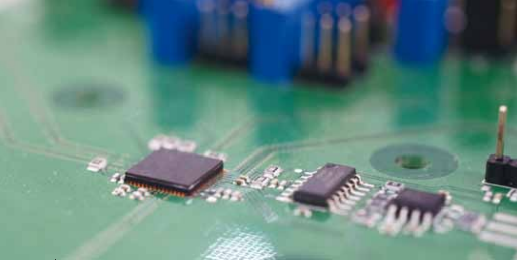
06 | Test PCB with imec and Holst Centre's wake-up receiver
