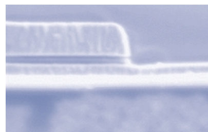
1.1\text{ fF/mm}^2 double metal capacitor.
