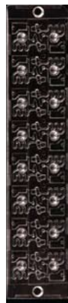
Microfluidic plastic chip for measuring droplets down to 0.5 \mu\text{L} .
