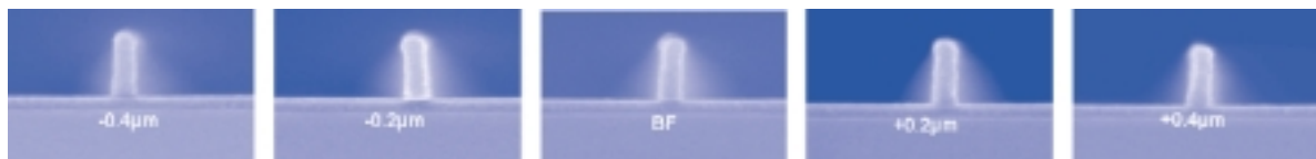
70-nm lines printed through focus using the ASML PAS5500/900 ArF step and scan system.
