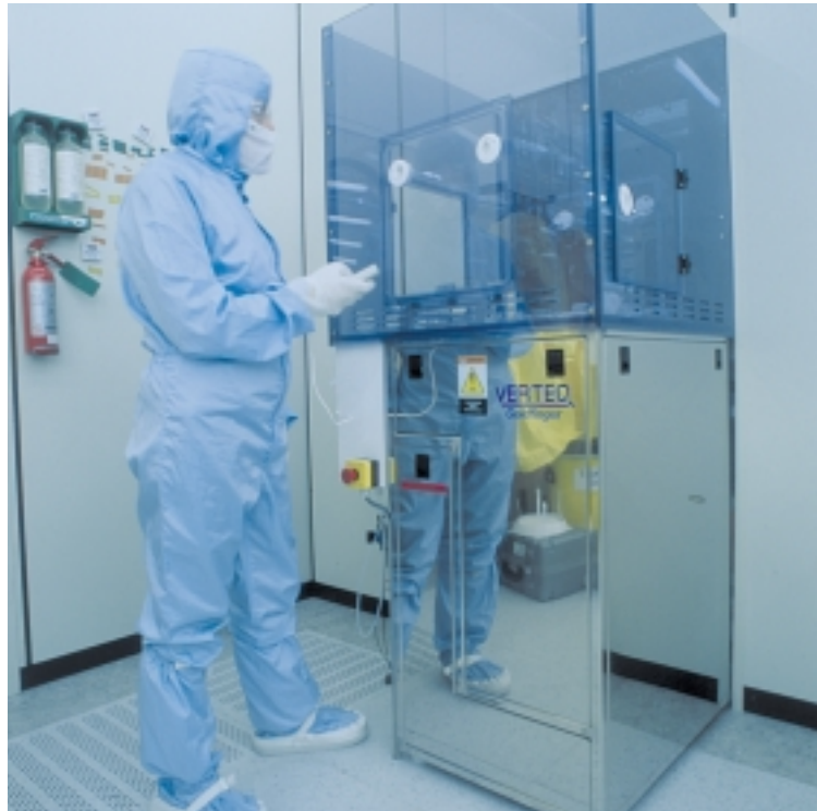
Goldfinger megasonic single-wafer-cleaning module
